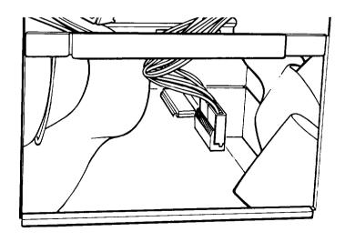
7. Lift the entire subassembly out of the computer and carefully place it on your work surface.
